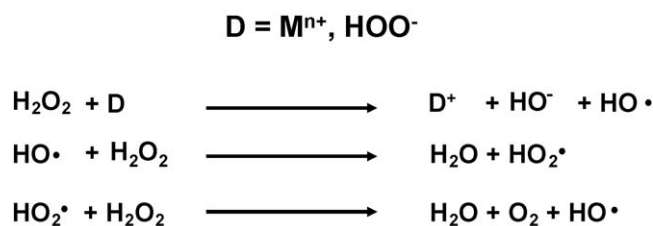
Scheme 5. A radical chain model for \text{H}_2\text{O}_2 decomposition. Conceivable donors, D are \text{M}^{n+} cations in diverse oxidation states and \text{HOO}^- (see text).
